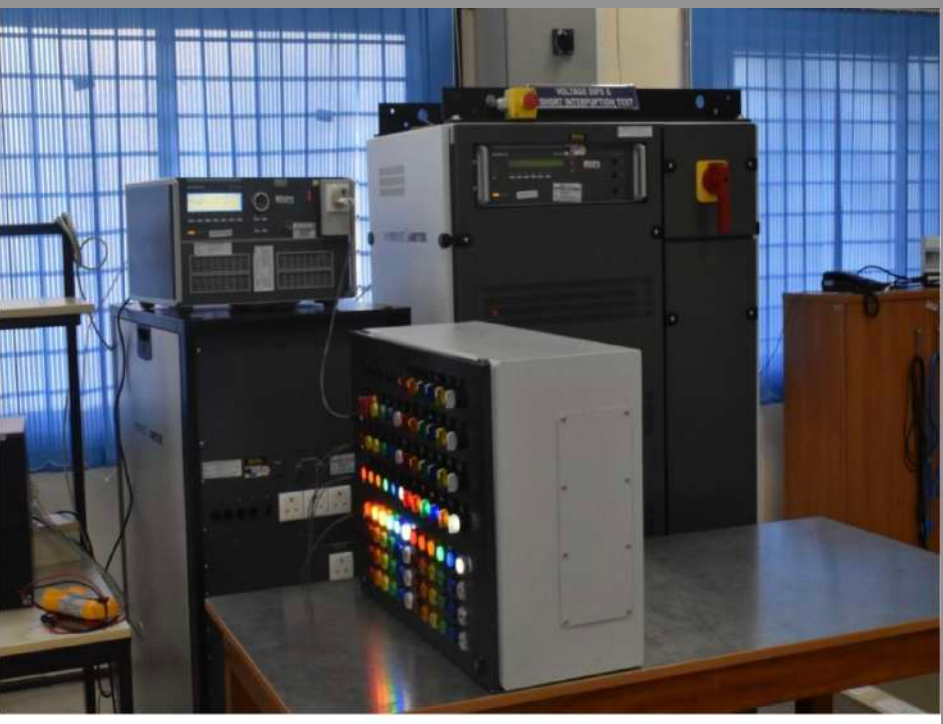
Voltage Dips & Short Interruptions Test Setup
