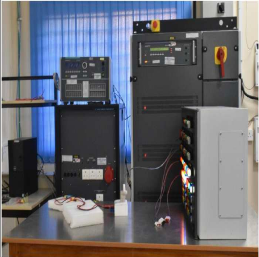
Harmonics and Interharmonics Test Setup
