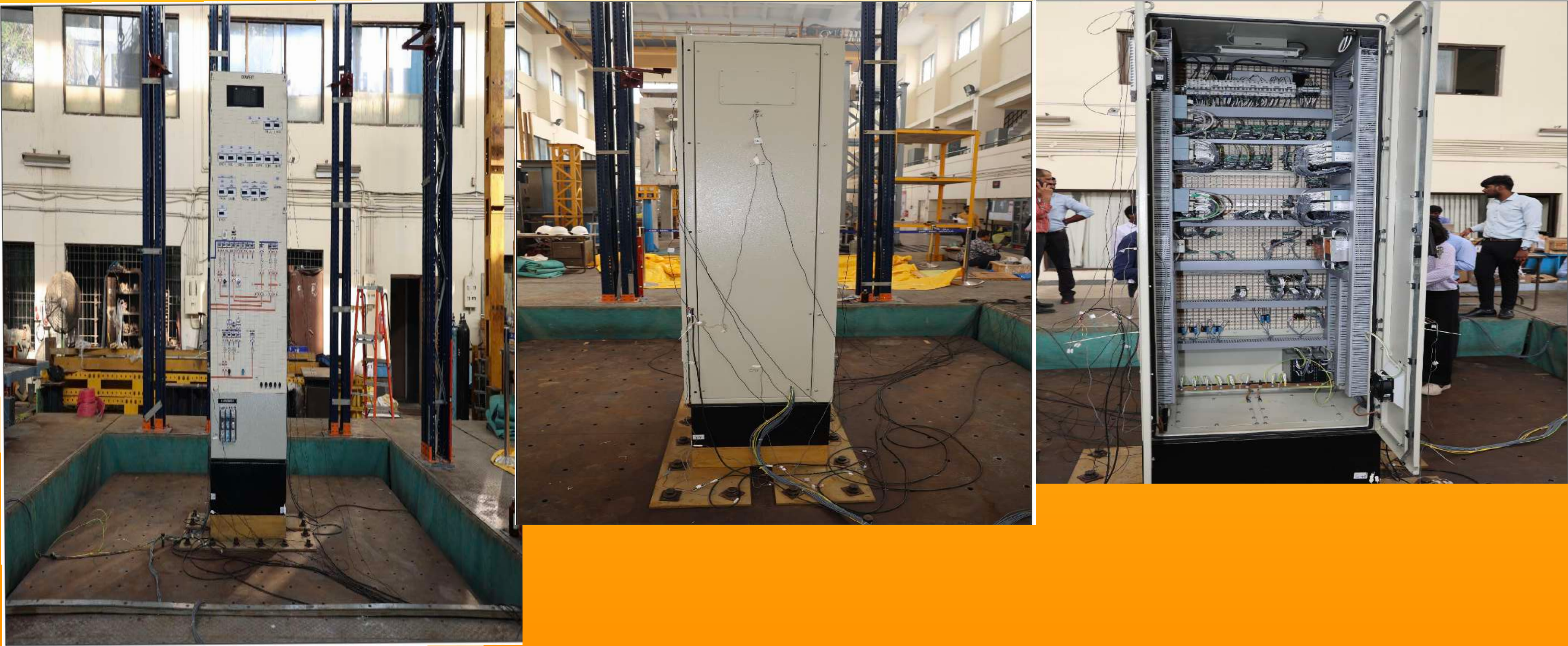
Fig. 1 Front view of the Mosaic Panel Board mounted on shake table
